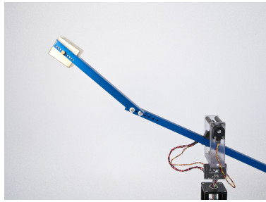
Figure 3.6: Connect the 3 DOF Helicopter tail.
