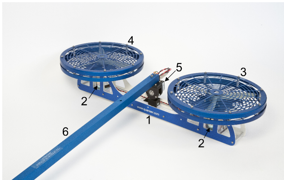
Figure 2.3: Components on the helicopter body of the 3 DOF Helicopter system.
