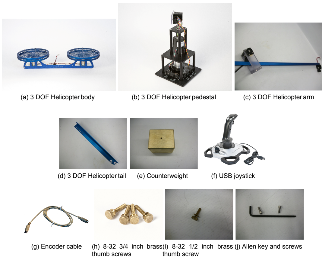
Figure 3.1: 3 DOF Helicopter components.
