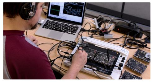
The AELabs is a series of modular boards that traverses the most important concepts in modern analog electronics.
