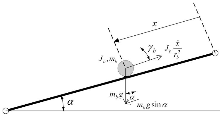
Figure 2.3: Completed Ball and Beam free-body diagram.
