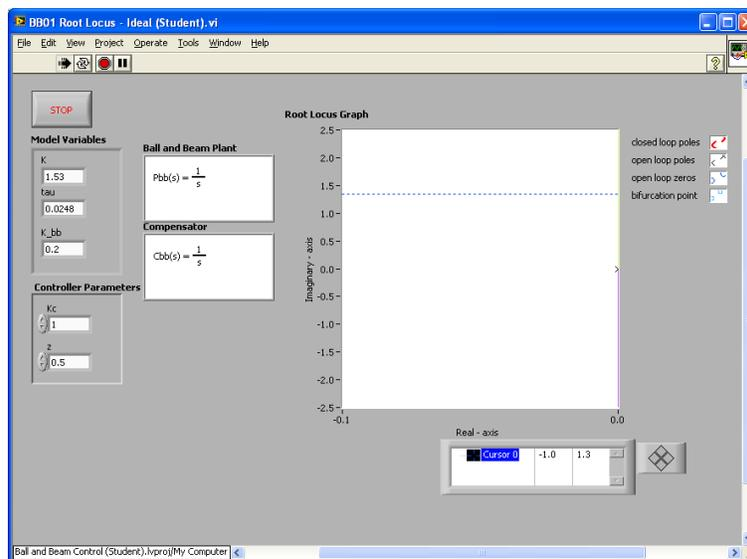
Figure 4.1: VI used to plot root locus of BB01 system with ideal control.
