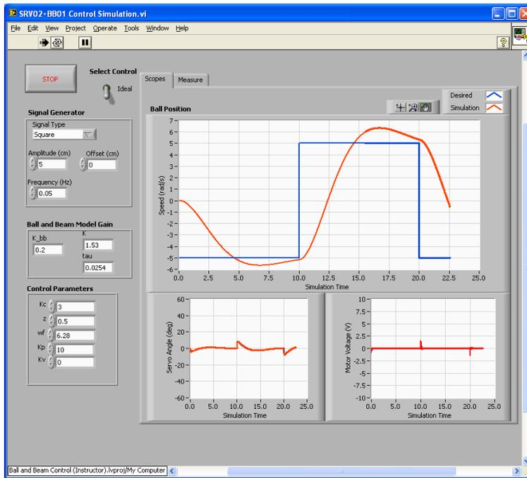
Figure 4.4: VI used to simulate cascade control system.
