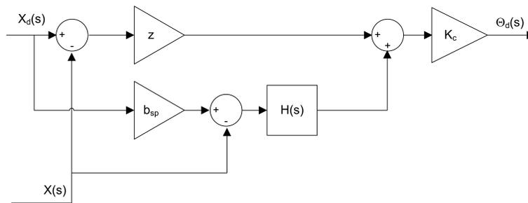
Figure 2.8: BB01 practical PD controller with filtering.
