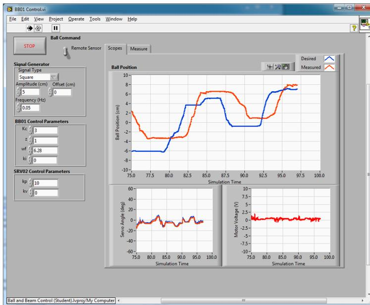
Figure 4.6: BB01 ball position response with SS01.
