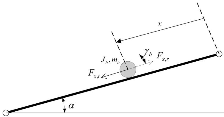
Figure 2.2: Free-body diagram of Ball and Beam.
