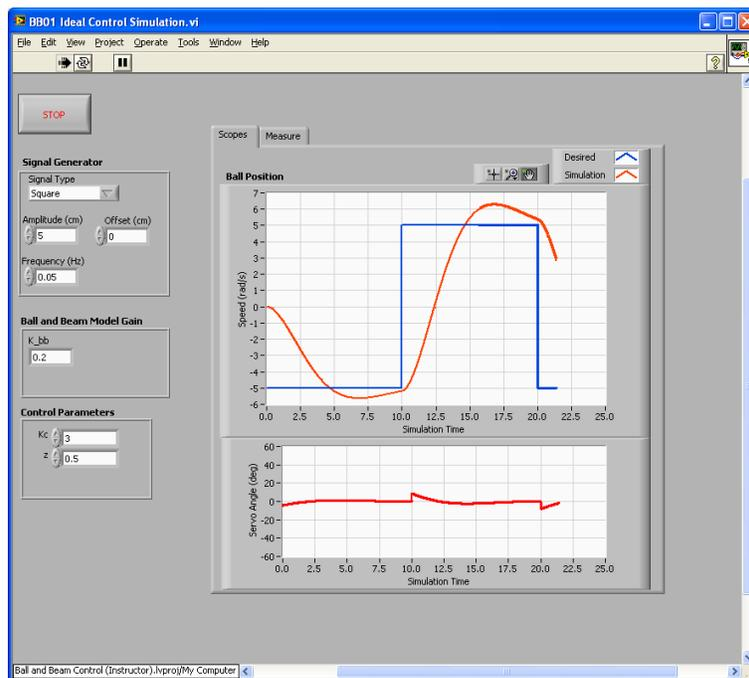
Figure 4.3: VI used to simulate the outer closed-loop BB01 system.
