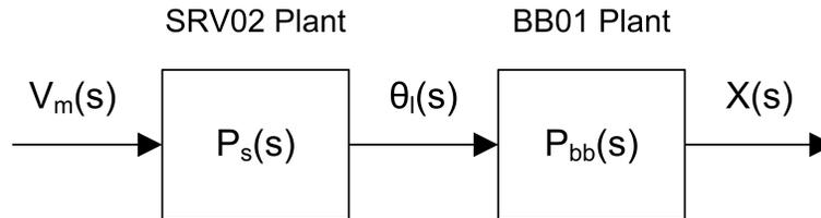
Figure 2.1: Ball and Beam open-loop block diagram.
