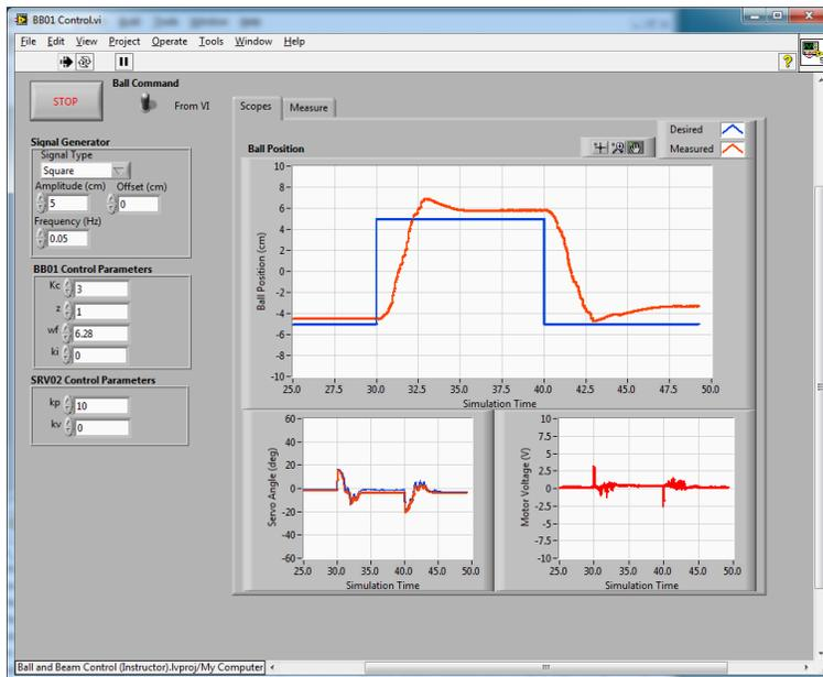
Figure 4.5: VI that runs the practical PD controller on the Ball and Beam system.
