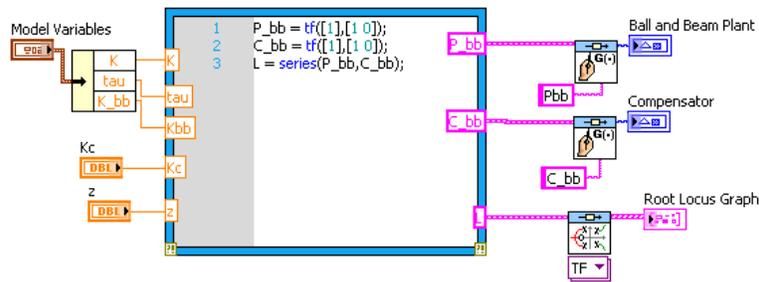
Figure 4.2: MathScript used to generate ideal loop transfer function of BB01 system (incomplete).
