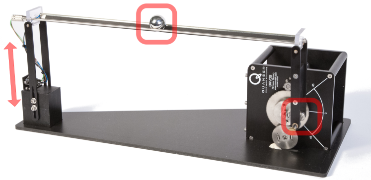
Figure 4.4: Adjust height of support column until ball is balanced at middle of beam
