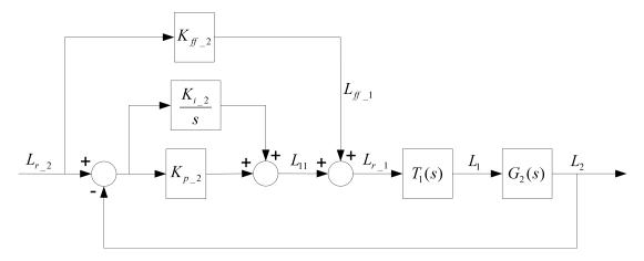
Figure 4.1: Tank 2 Water Level PI-plus-Feedforward Control Loop.
