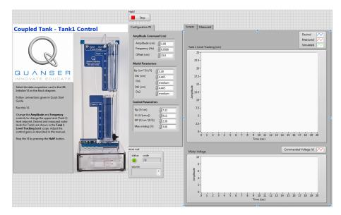
Figure 3.5: VI used to run PI-FF control on Coupled Tanks system in configuration #1.
