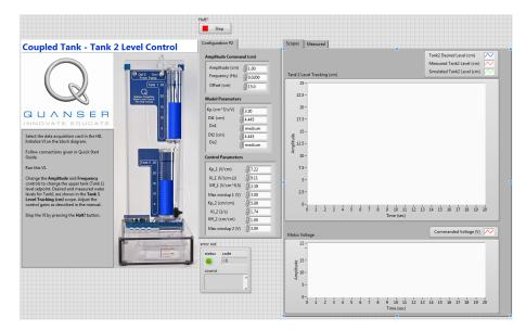
Figure 4.3: VI used to run PI-FF control on Coupled Tanks system in configuration #2.
