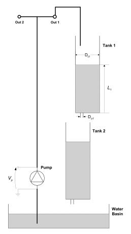
Figure 2.1: Schematic of Coupled Tank in Configuration #1.
