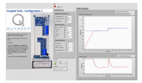
Figure 3.4: VI used to run PI-FF control Simulation on Coupled Tanks system in configuration #1.
