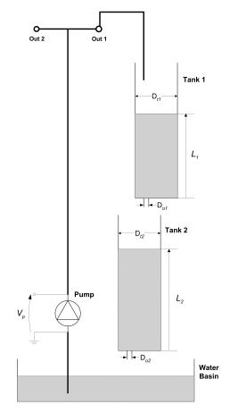
Figure 2.2: Schematic of Coupled Tank in configuration #1.
