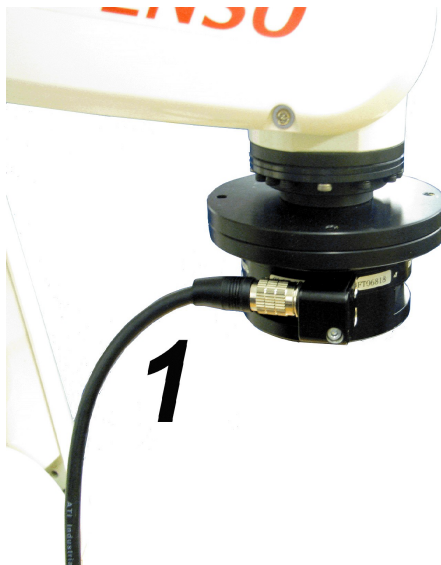
Figure 4.5: Force-torque sensor on Denso arm
