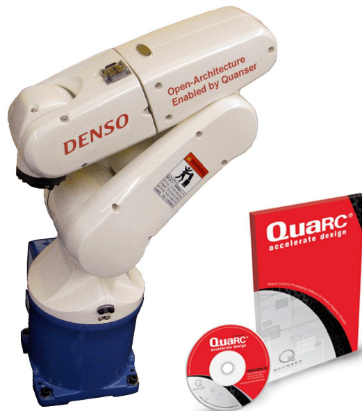
Figure 1.1: The open-architecture 6-axis robot enabled by Quanser
