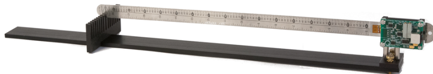
Figure 4.6: Mounting Flexible Pendulum on calibration base.
