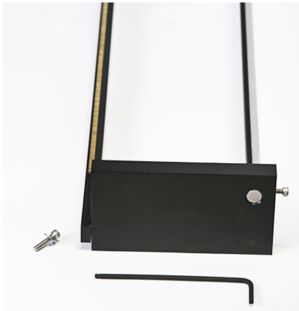
Figure 4.1: Remove the rack end plate
