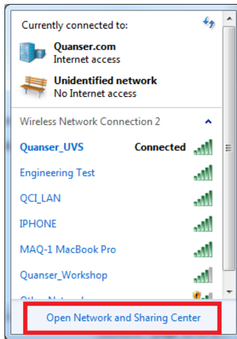
Figure 3.1: Open network settings. The Unidentified network is related to the wired connection to the router. If you are using a wired connection to the router and you don't have wireless adapter, you will not see Quanser_UVS network.
