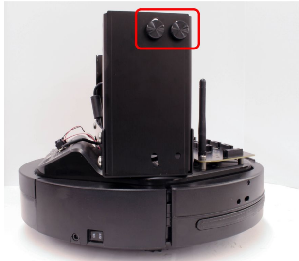
(b) The QBot 2 Kinect thumb screws
