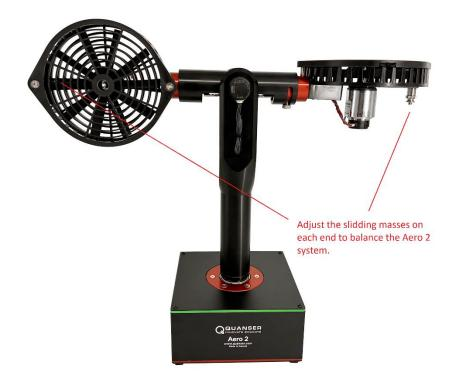
Figure 6. Mass sliders for leveling the Aero 2 unit
