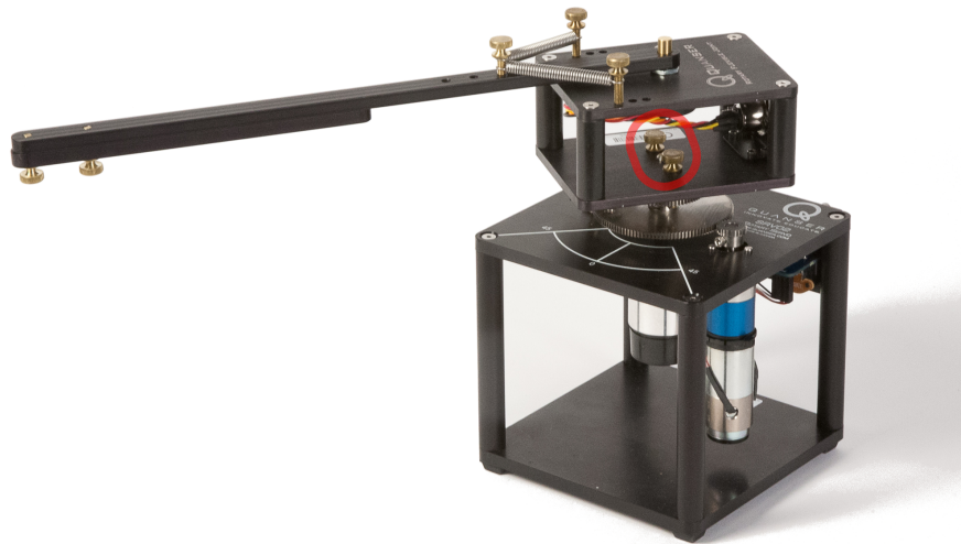
Figure 4.1: Attach ROTFLEX to SRV02 using thumb screws
