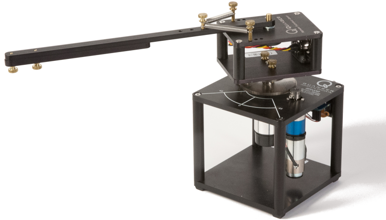
Figure 1.1: Rotary Flexible Joint system
