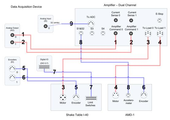
Figure 3.1: Shake Table I-40 Connections when using One-Floor Active Mass Damper
