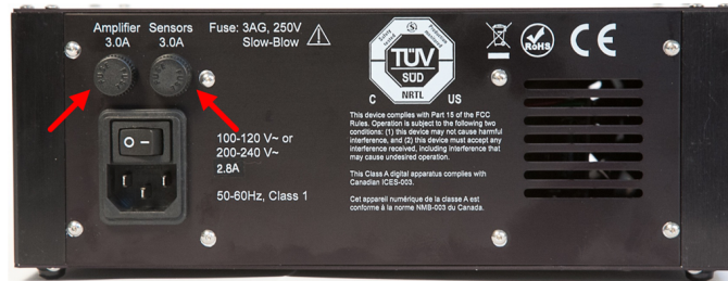
Figure 4.1: VoltPAQ-X1 fuse holders
