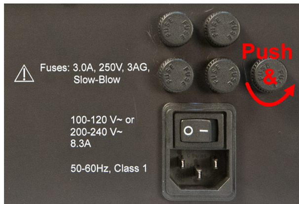
Figure 4.1: Remove fuse holders (VoltPAQ-X4 shown)
