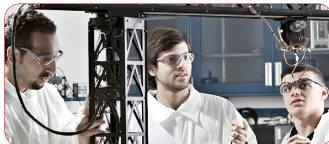
Mechanical engineering students from Texas A & M University at Qatar use the 3 DOF Crane workstation in their lab to understand the dynamics and control challenges in everyday crane operation.
