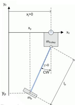
Figure 1. Linear gantry challenge teaches how to minimize payload swings as the trolley move across the jib.
