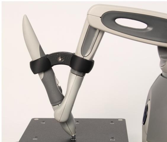
Figure 1.4: Custom configuration of the stylus
