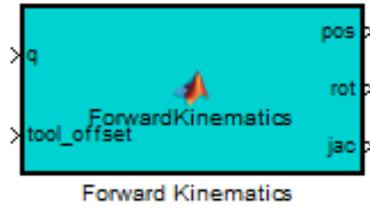
Figure 8.2: Forward kinematics block with jacobian
