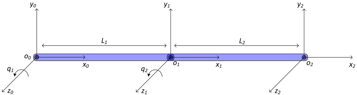
Figure A.1: Two-link planar elbow
