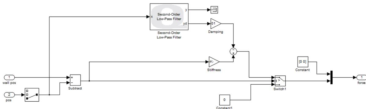
Figure 11.3: Wall force model subsystem
