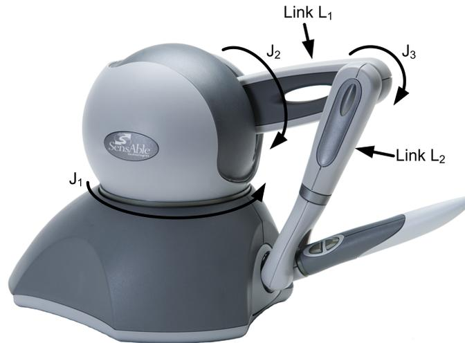
Figure 1.2: The three actuated joints on the Omni<sup>1</sup>
