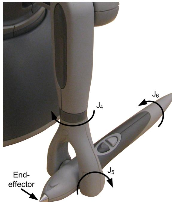
Figure 1.3: Non-actuated joints and the end-effector<sup>1</sup>
