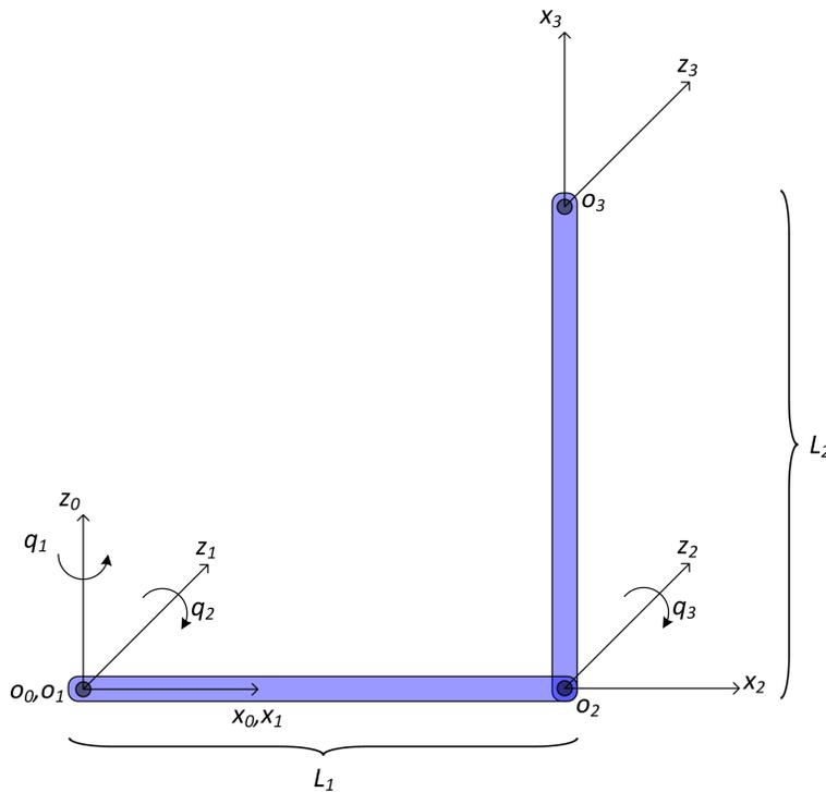
Figure 3.1: Coordinate frames to get the D-H parameters
