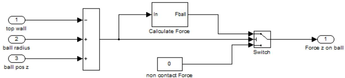
Figure 12.4: **PD Contact Top Wall** model
