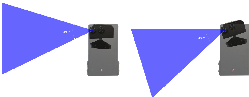
Figure 2.3: Relative FOV of the tilted Kinect sensor
