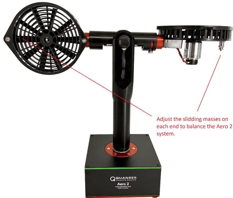
Figure 6. Mass sliders for leveling the Aero 2 unit
