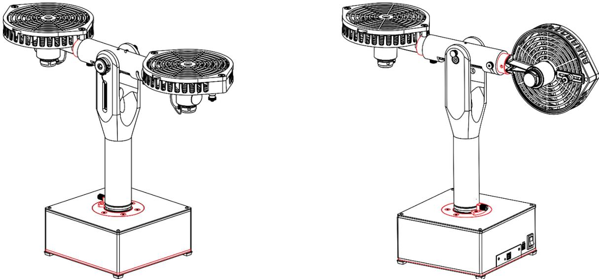
Half-Quad configuration (pitch locked, yaw free), or
