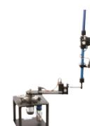
Rotary Double Inverted Pendulum
