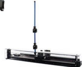
High Fidelity Linear Cart with Triple Inverted Pendulum
