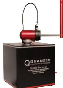
Encoder angle sensed inverted pendulum
