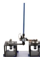
2 DOF Inverted Pendulum
