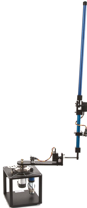
Figure 1.1: Quanser Double Inverted Pendulum (DBPEN-ROT).
