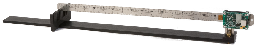
Figure 4.5: Mounting FLEXGAGE on calibration base.
