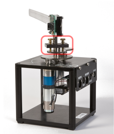
Figure 4.1: Mounting the FLEXGAGE onto the SRV02
