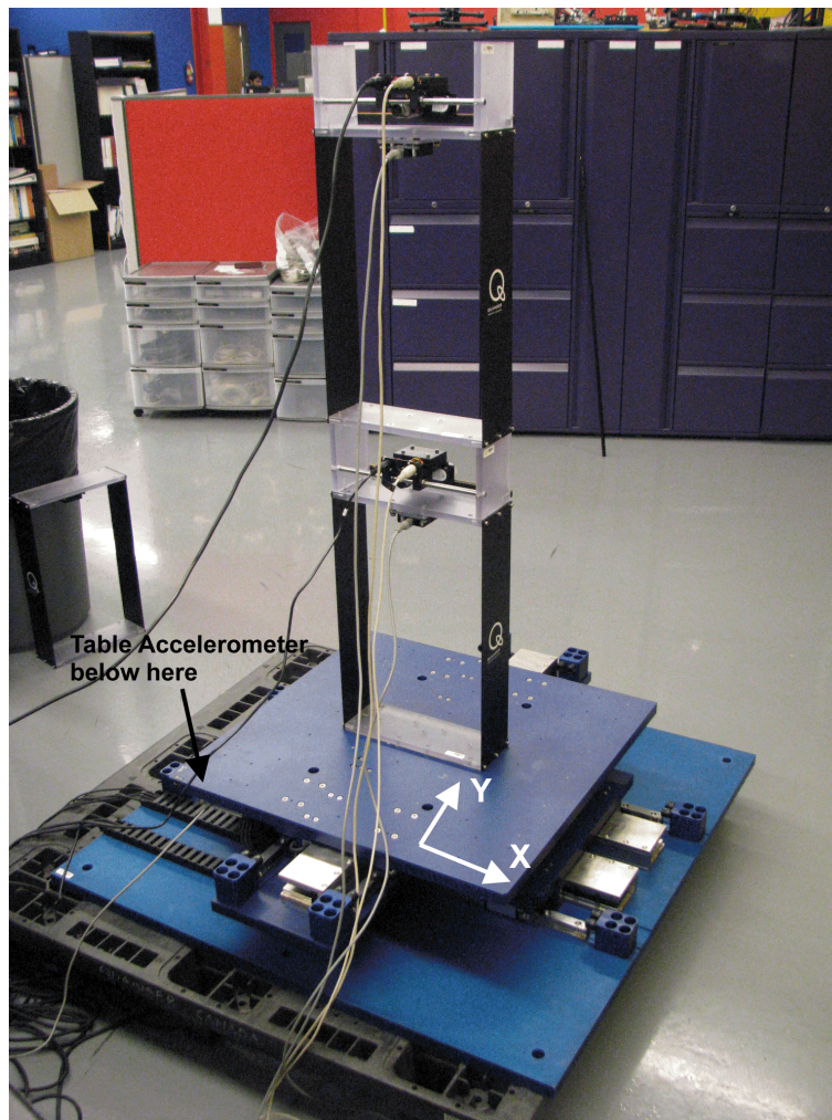
Figure 3.2: Two-Floor Active Mass Damper on XY Shake Table III
